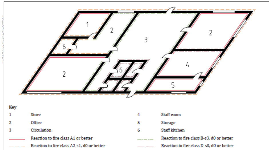
Figure C.11 — Example of fire safety information as represented in information deliverables – Reaction to fire requirement
