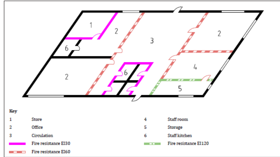
Figure C.10 — Example of fire safety information as represented in information deliverables – Fire resistance requirement
